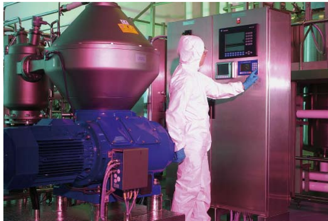
Fig. 3: A large scale intermittent discharge continuous centrifuge as used in cGMP manufacture.
